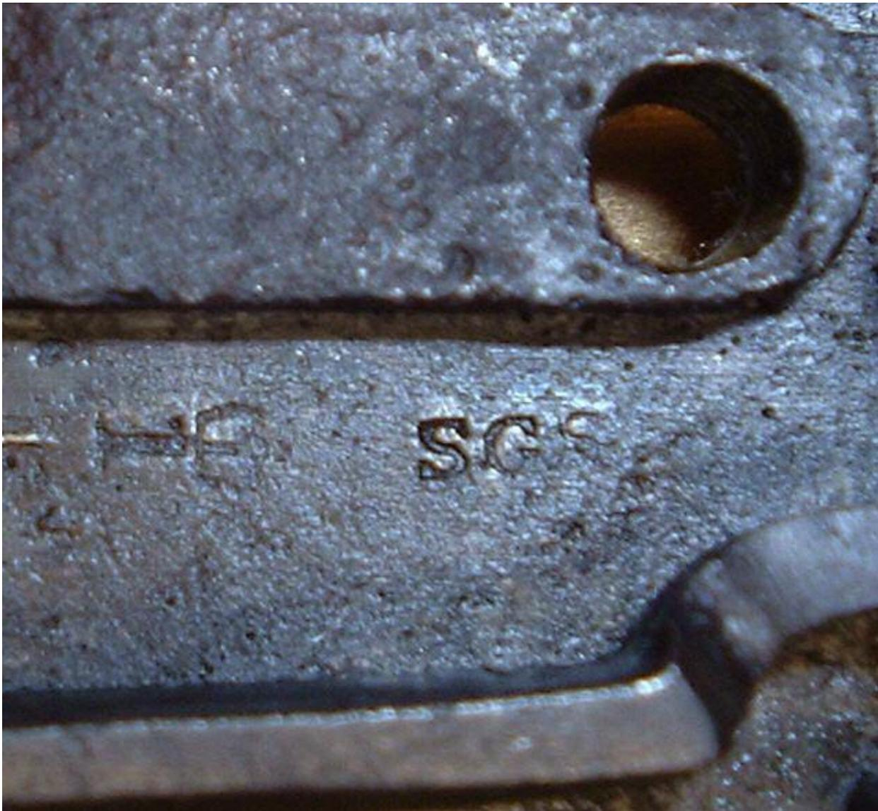
**Figure 2. Apparently mis-struck SGS mark.**
