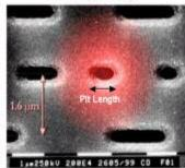
Track Pitch: 1,6 micron Minimum Pit Length: 0,8 μm Storage Density: 0,41 Gb/inch<sup>2</sup>
