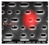
Track Pitch: 0,74 micron Minimum Pit Length: 0,4 μm Storage Density: 2,77 Gb/inch<sup>2</sup>
