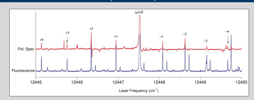
Comparison excitation scan showing both polarization spectroscopy (top) and laser-induced fluorescence spectroscopy (bottom) Direct pump-probe transition is
