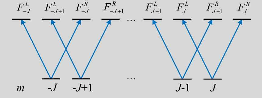
Polarization signal depends on the difference of absorption between left and right circular polarization components of the linearly polarized probe beam
