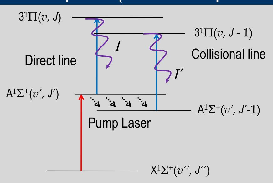
Ratio of fluorescence intensities is roughly equal to the ratio of population densities in the collisionally and directly populated level
